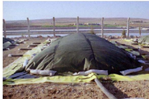
Figure 13c: Biological rotting under a semipermeable membrane
