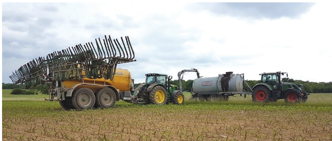
● Fig. 11: Pumping the liquid manure from the transportation tank to the spreading tank
