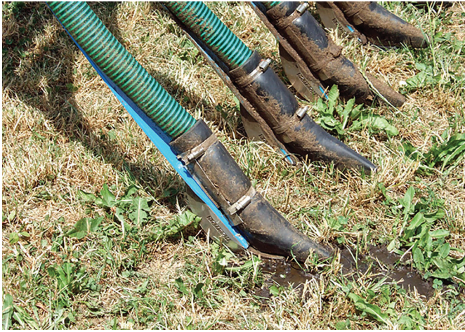
Fig. 15: Trailing shoe in details
