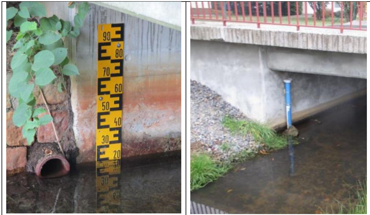
Figure 4: Examples of Water Level Gauges for Surface Water
