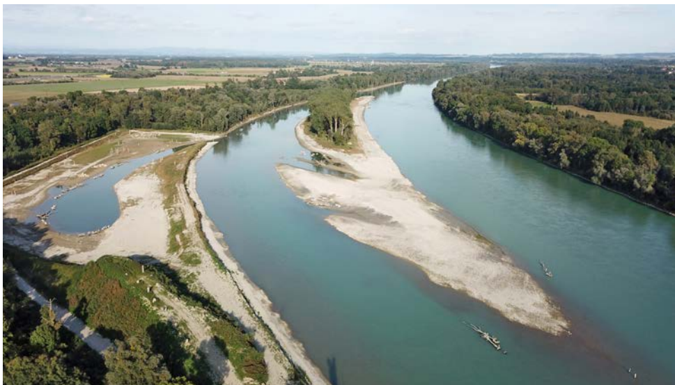
Larger gravel island and newly connected tributary in a restored Inn river stretch directly downstream of a hydropower barrag
