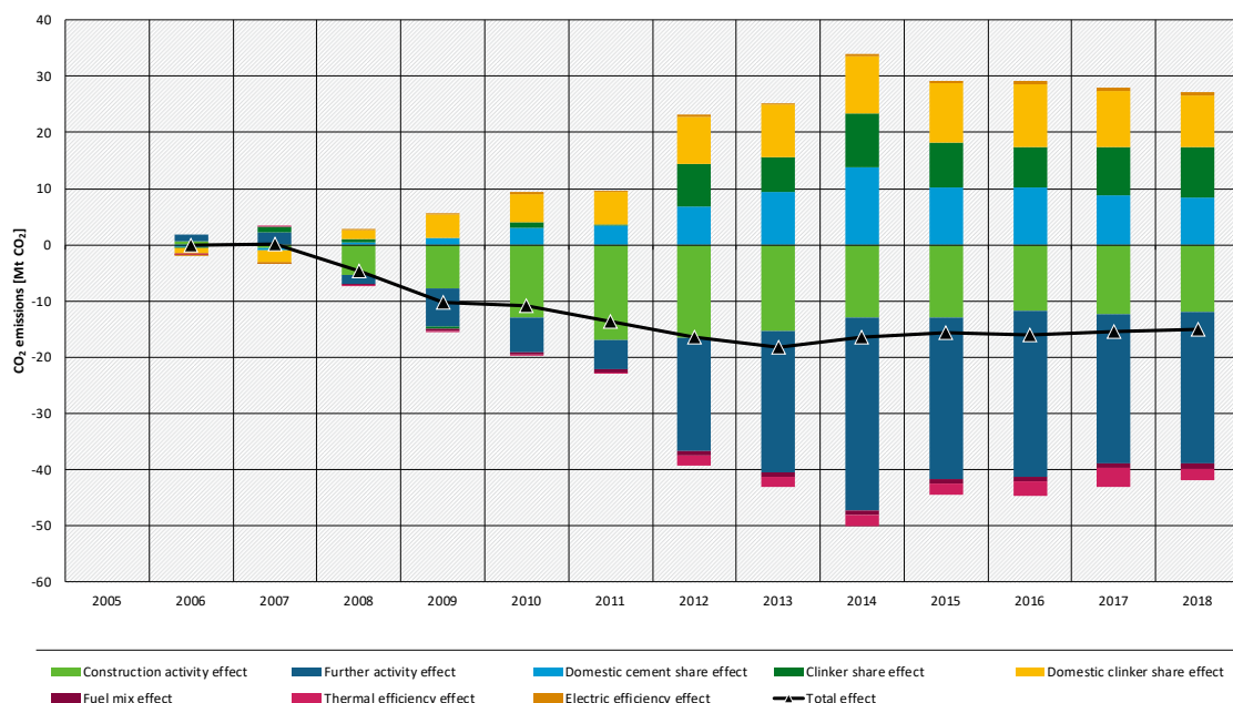
Figure 6: Decomposition of the development of CO 2 emissions from cement production since 2005 in Spain
