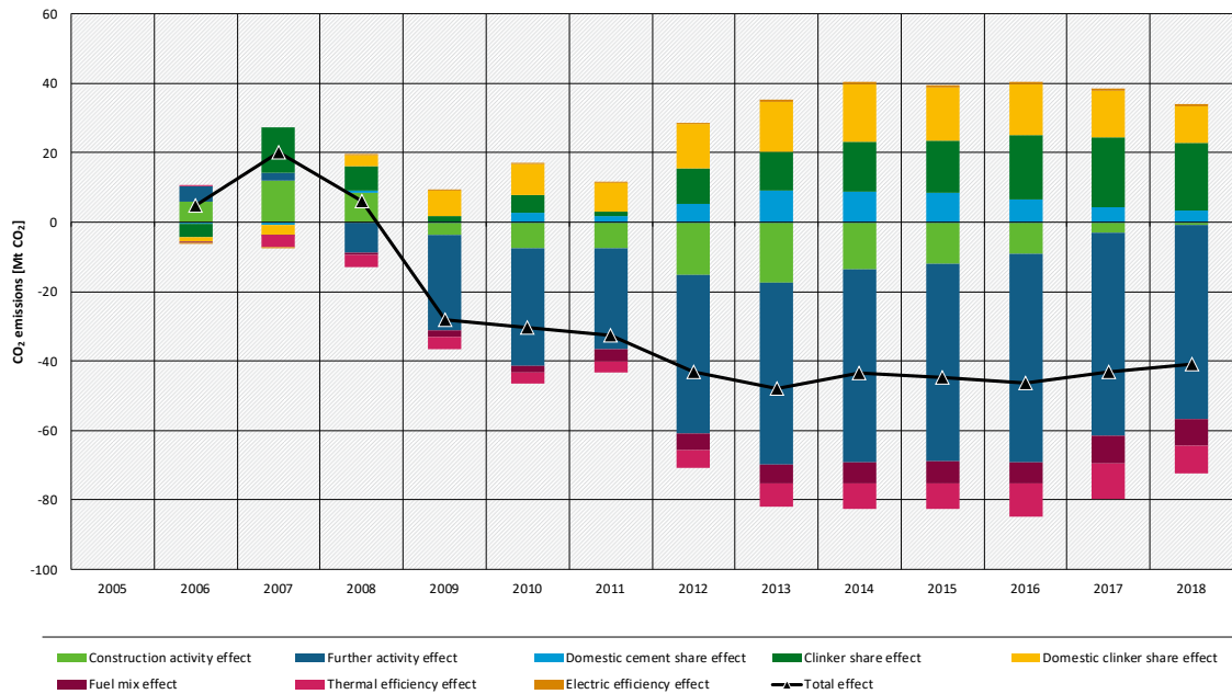
Figure 4: Decomposition of the development of CO 2 emissions from cement production since 2005 in the EU28
