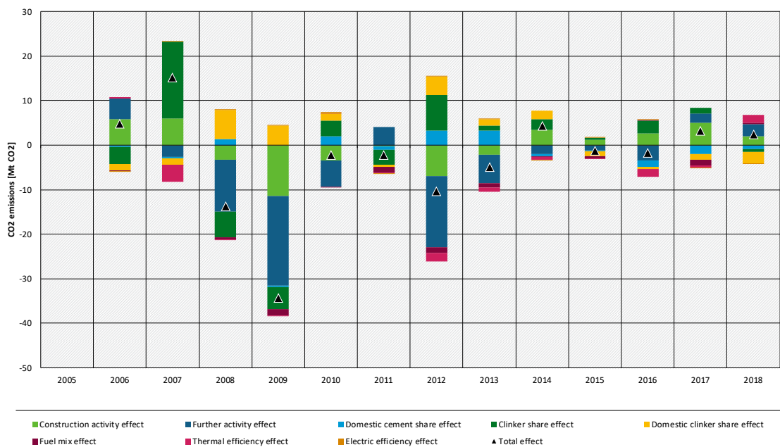
Figure 5: Decomposition of the annual change of CO 2 emissions from cement production in the EU28
