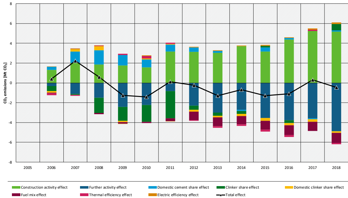
Figure 12: Decomposition of the development of CO 2 emissions from cement production since 2005 in Germany
