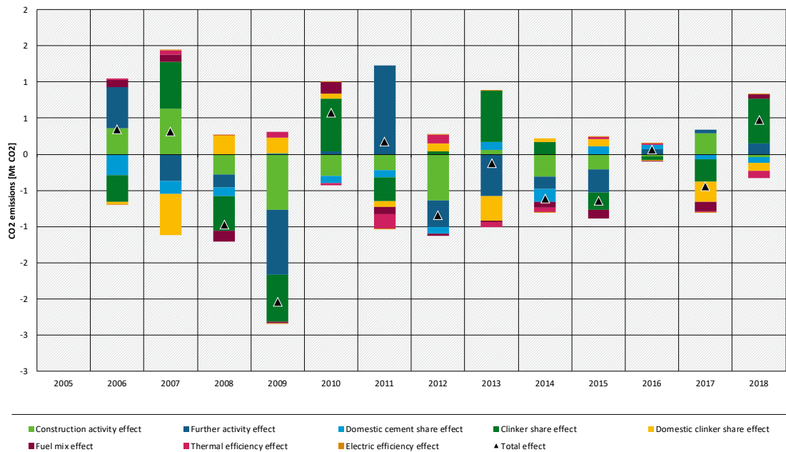
Figure 11: Decomposition of the annual change of CO 2 emissions from cement production in France
