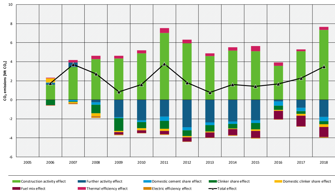
Figure 14: Decomposition of the development of CO 2 emissions from cement production since 2005 in Poland
