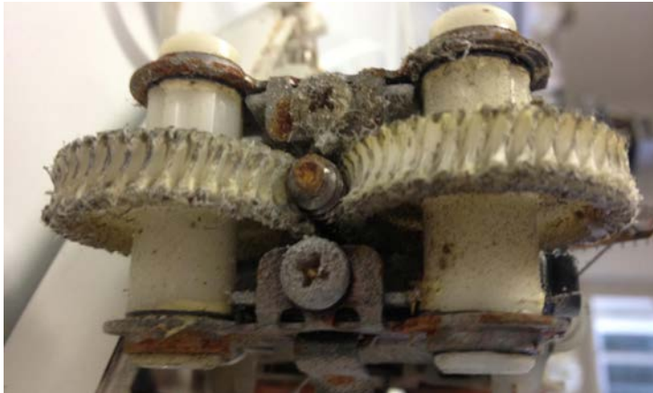
Figure 85 Example of worn cog-wheels of a hand mixer
