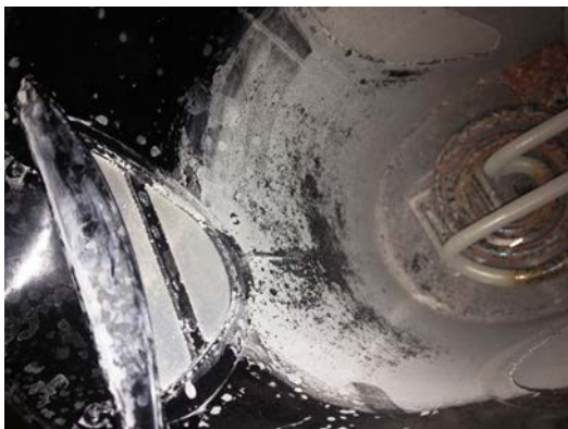
Figure 86 Scaling in a kettle
