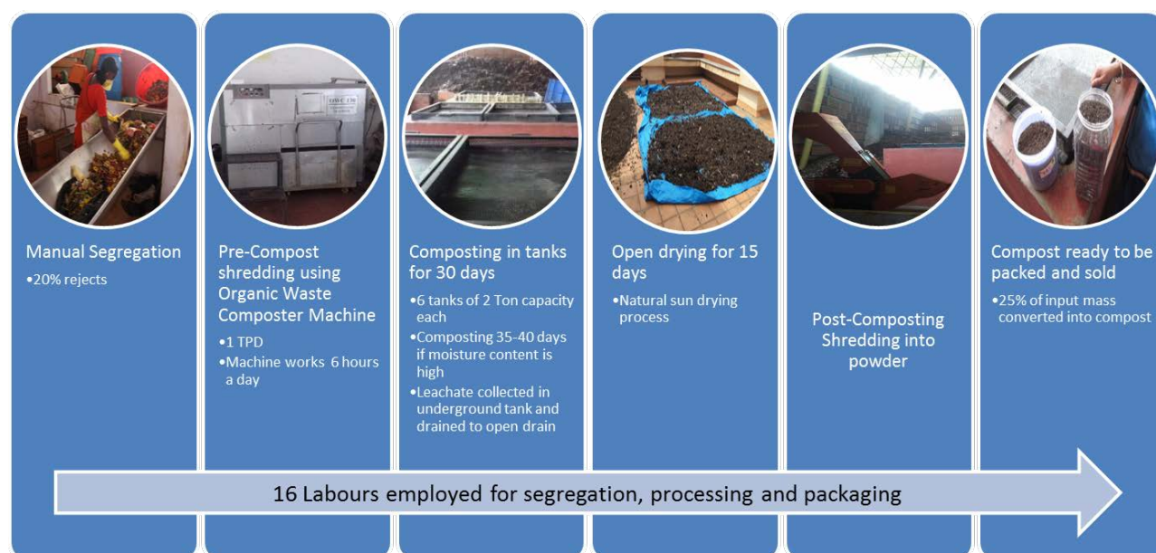
Figure 15: Composting process Ward No 151
