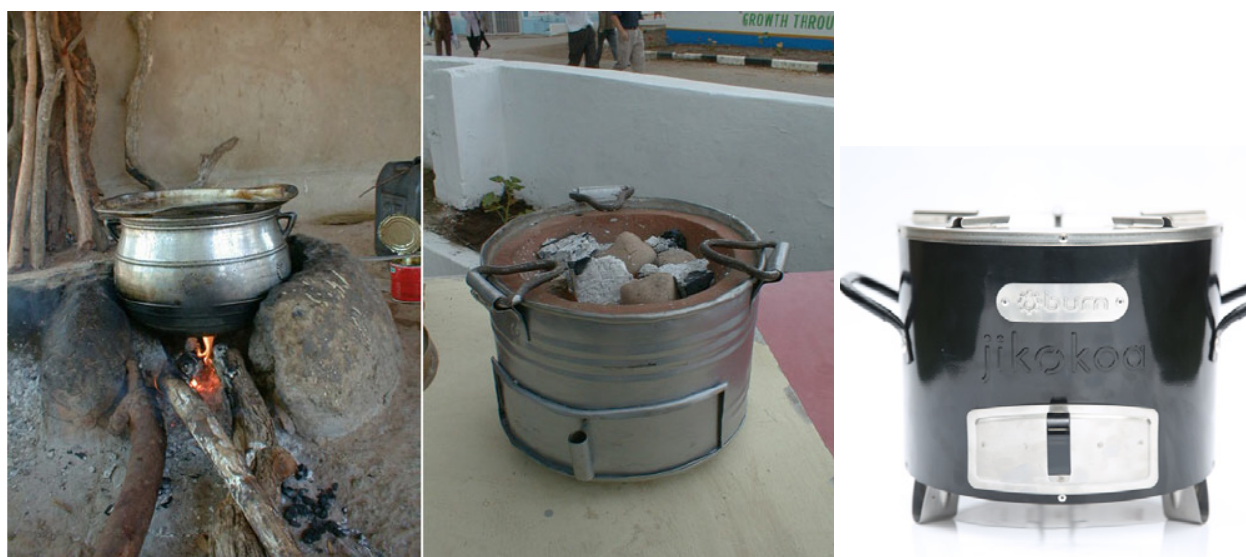
Figure 17: Comparison of wood, charcoal, and ethanol cookstove types
