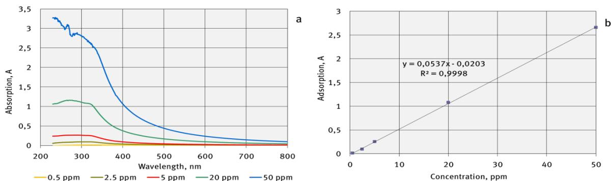
Figure 14: UV-VIS spectra obtained while testing the dispersions of TiO<sub>2</sub> (NM105) with concentrations (a) 0.5-50 ppm in presence of 30 ppm DOC and (b) calibration line based on obtained spectra, (optimal wavelength of 300nm)
