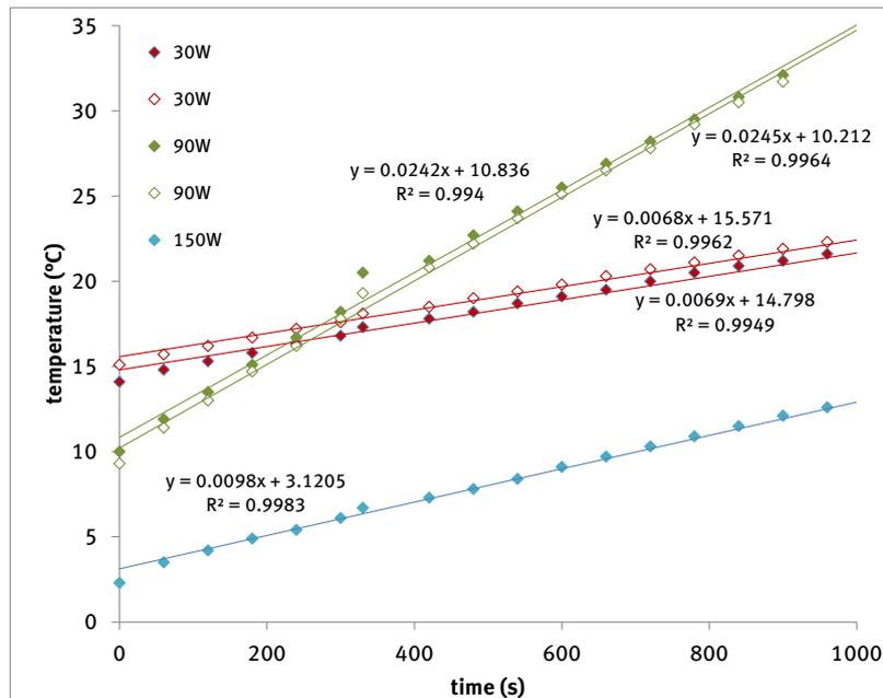
Figure 7: Calibration of delivered acoustic energy during sonication. Determination of slope of the linear trend line fit.
