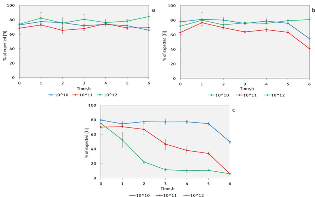
Figure 25: Agglomeration behavior of  $\text{TiO}_2$  (NM105) nanoparticles in the dispersions of various particle number concentrations:  $10^{10}$ ,  $10^{11}$ ,  $10^{12}$  particles /L. (a) in MQ, (b) in 1 mM  $\text{Ca}(\text{NO}_3)_2$  and (c) in 5 mM  $\text{Ca}(\text{NO}_3)_2$ .
