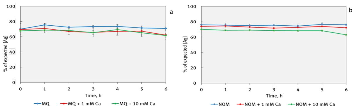
Figure 19: Agglomeration behavior of Ag (NM300K) nanoparticles. (a) in 0, 1, 10 mM Ca(NO<sub>3</sub>)<sub>2</sub> media, (b) in 0, 1, 10 mM Ca(NO<sub>3</sub>)<sub>2</sub> and 30 ppm DOC (SRNOM) media. Error bars from 3 replicate experiments.
