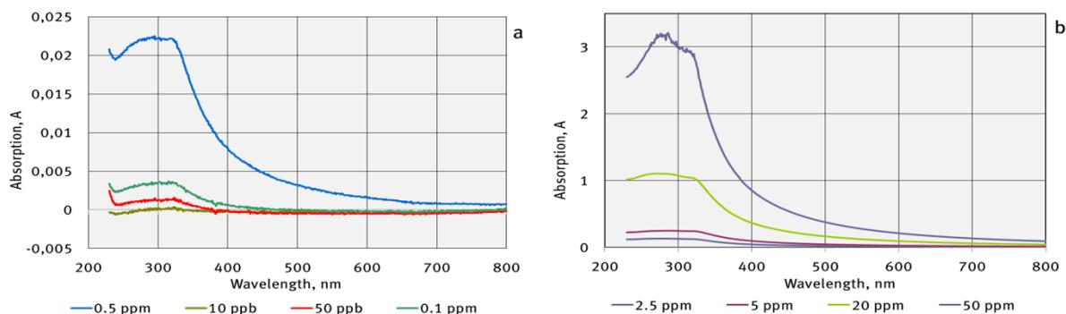
Figure 12: UV-VIS spectra obtained while testing the dispersions of TiO<sub>2</sub> (NM105) with concentrations of (a) 0.01-0.5 ppm and (b) 2.5-50 ppm
