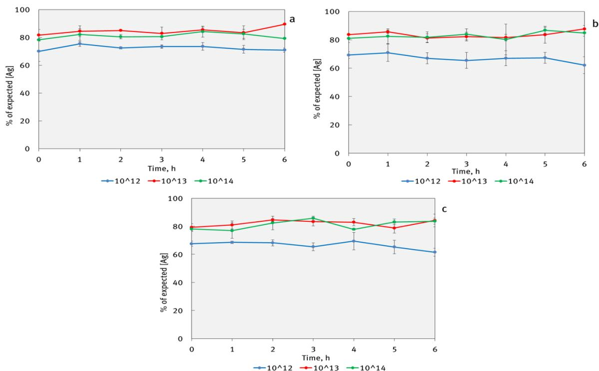
Figure 26: Dispersion stability of Ag (NM300K) particles in the dispersions of various density: 10<sup>12</sup>, 10<sup>13</sup>, 10<sup>14</sup> particles /L. (a) in MQ, (b) in 1 mM Ca(NO<sub>3</sub>)<sub>2</sub> and (c) in 5 mM Ca(NO<sub>3</sub>)<sub>2</sub>.
