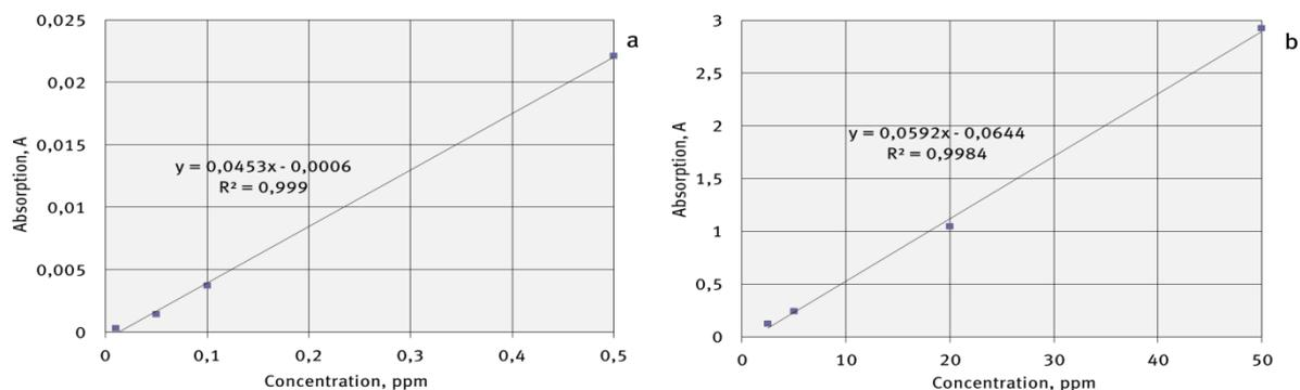
Figure 13: Calibration functions obtained based on the UV-VIS spectra. (a) 0.01-0.5 ppm and (b) 2.5-50 ppm of TiO<sub>2</sub> (NM105) in MQ (without DOC). At optimal detection wavelength of 300 nm
