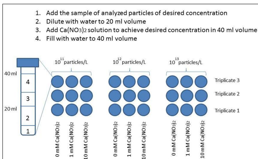
Figure 6: Possible experimental design to investigate nanoparticle dispersion behavior in dispersions with various particle concentrations.
