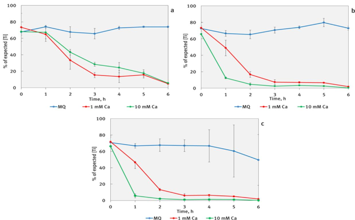
Figure 23: Agglomeration behavior of TiO<sub>2</sub> (NM105) nanoparticles at pH=8.5. pH values were established in presence of (a) 1 mM NaHCO<sub>3</sub>, (b) 5 mM NaHCO<sub>3</sub>, (c) 10 mM NaHCO<sub>3</sub> and the pH values remained stable during all experimental procedures.
