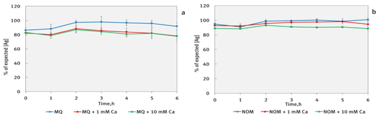
Figure 22: Agglomeration behavior of Ag (NM300K) nanoparticles in absence of CO<sub>2</sub>. (a) in 0, 1, 10 mM Ca(NO<sub>3</sub>)<sub>2</sub> media, (b) in 0, 1, 10 mM Ca(NO<sub>3</sub>)<sub>2</sub> and 30 ppm DOC (SRNOM) media.
