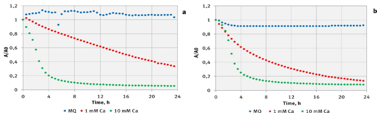
Figure 27: Dispersion stability of  $\text{TiO}_2$  particles in MQ media containing 0, 1 and 10 mM electrolyte (blue, red and green lines correspondingly). (a) at 380 nm wavelength. (b) at 600 nm wavelength.
