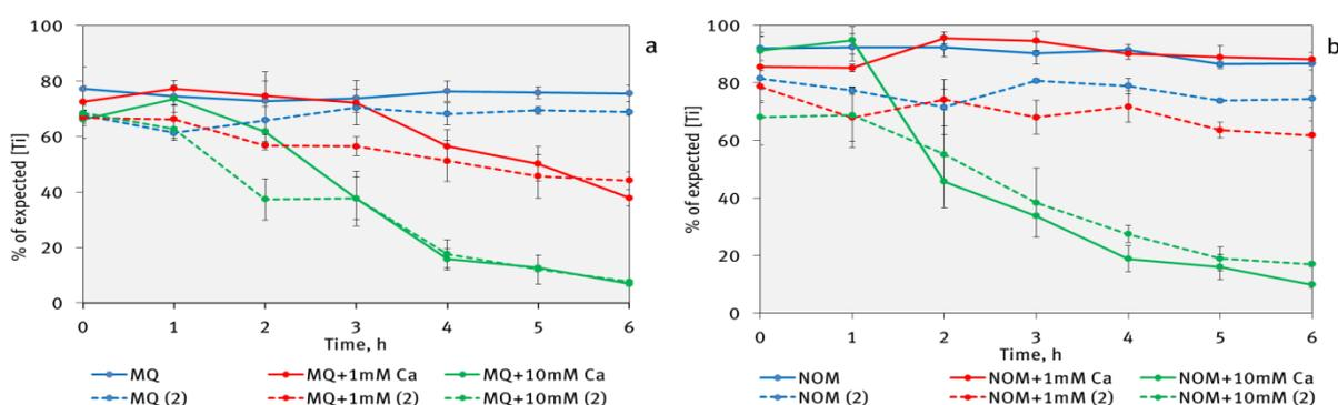
Figure 21: Agglomeration behavior of TiO<sub>2</sub> (NM105) nanoparticles in absence of CO<sub>2</sub>. (a) in 0, 1, 10 mM Ca(NO<sub>3</sub>)<sub>2</sub> media, (b) in 0, 1, 10 mM Ca(NO<sub>3</sub>)<sub>2</sub> and 30 ppm DOC (SRNOM) media. Replicate experiments marked with "(2)".
