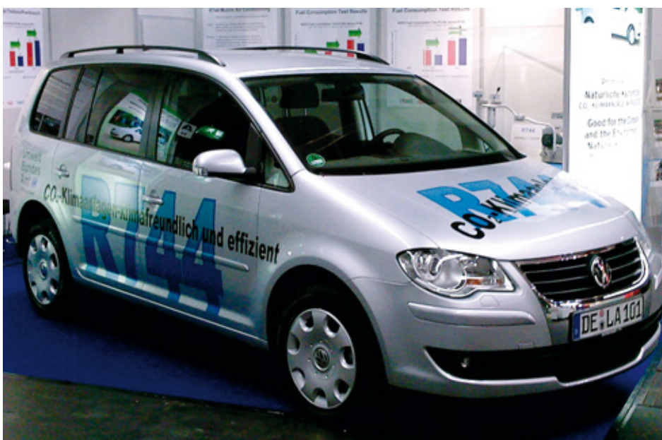
The UBA's official car with the CO 2 air conditioning system at the IAA trade show for commercial vehicles in 2008.
