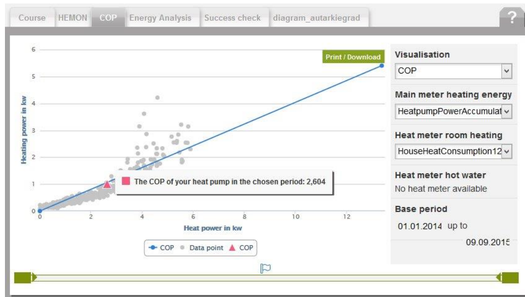
Figure 17: "Boiler signature" of a heat pump
