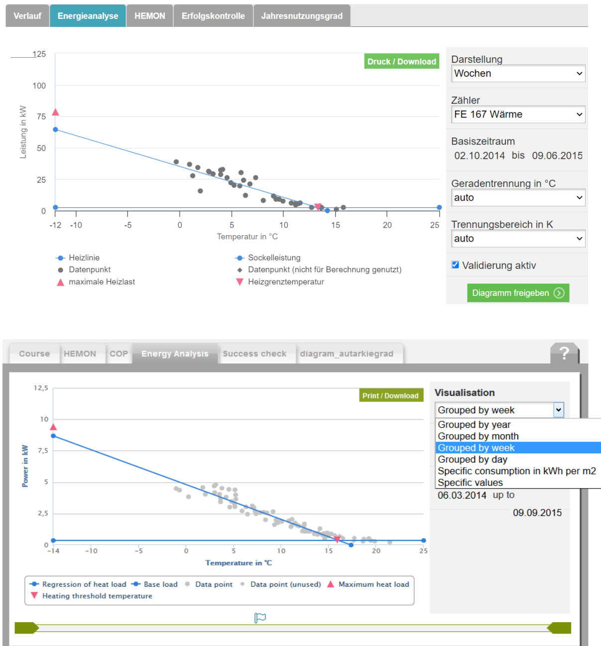
Figure 21: Energy analysis of boiler and heat pump in comparison
