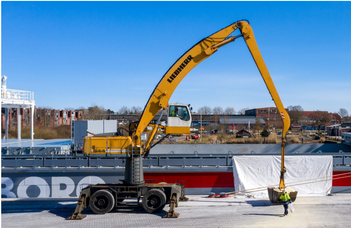
Figure 19 To prevent nutrients from entering the water, the space between the quay side and the ship is covered with a tarpaulin
