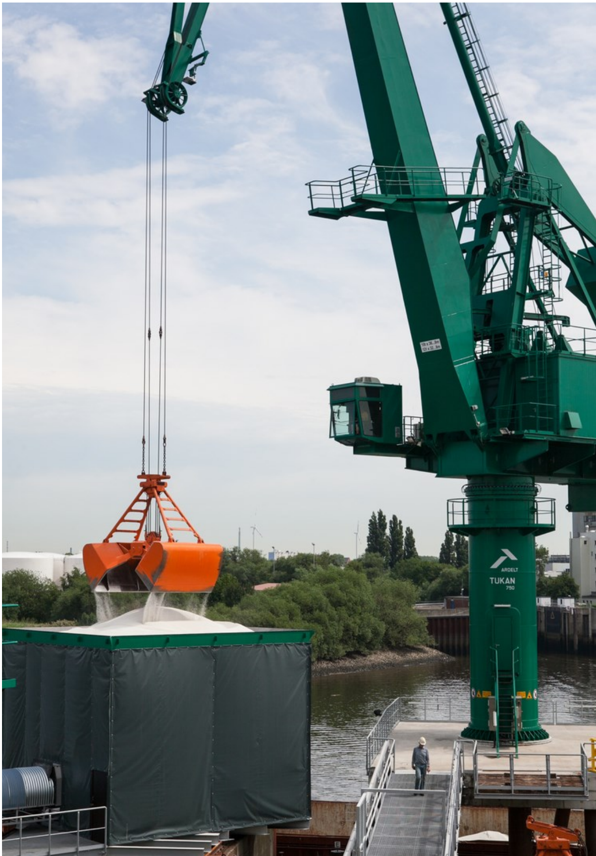
Figure 15 Rope hoist crane with closed bucket grab drops fertiliser into hopper
