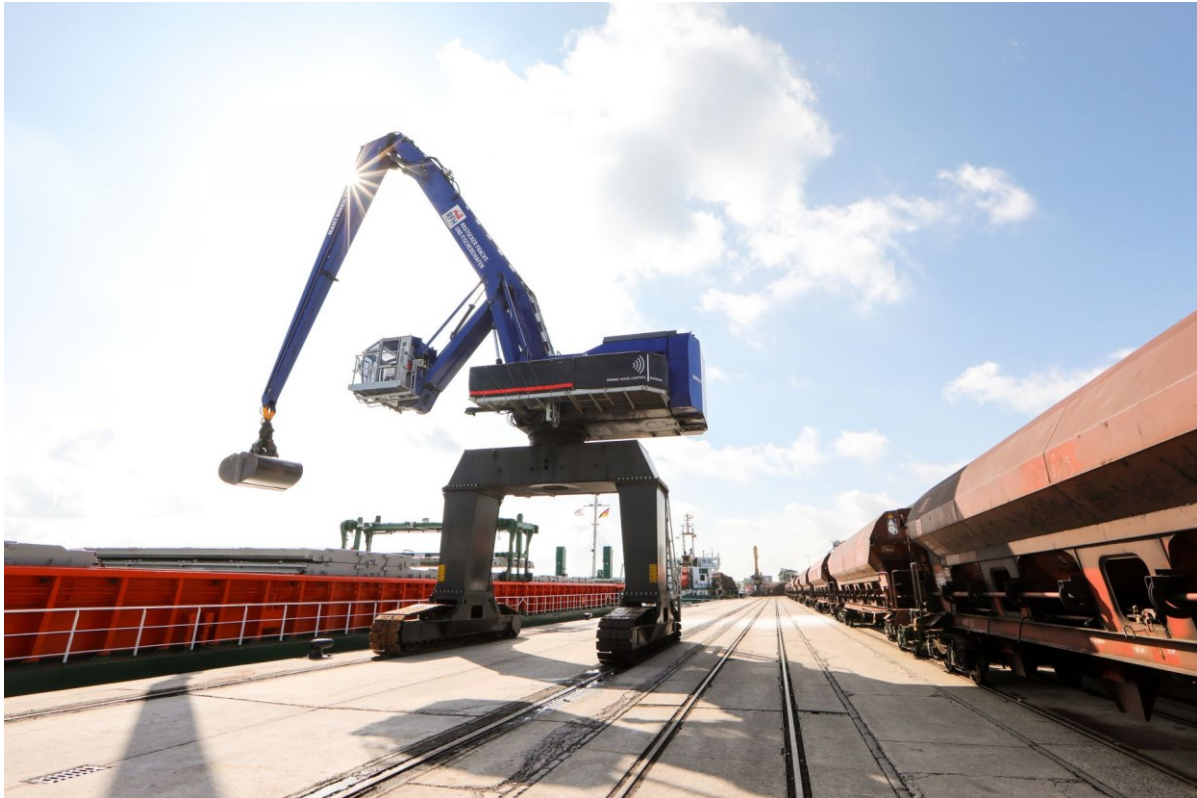
Figure 16 Port handling equipment Mantsinen 120R with articulated arm
