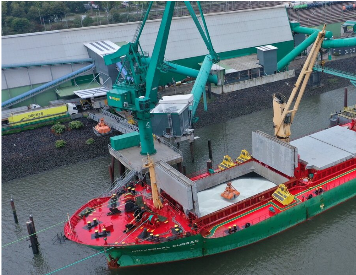
Figure 6 Unloading of a seagoing vessel by means of a closed grab bucket, discharge into hopper and storage by means of an enclosed conveyor belt
