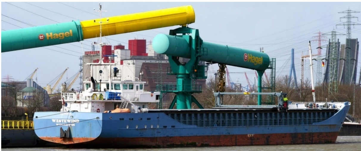
Figure 5 Ship loader and closed conveyor belt system during loading of an ocean-going vessel
