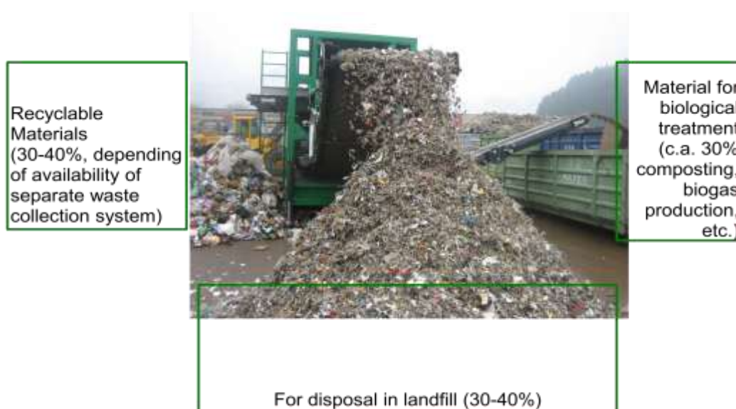
Fig. 6: Mechanical pre-treatment of the mixed municipal waste (Graph: A. Sirmais, Latvia)
