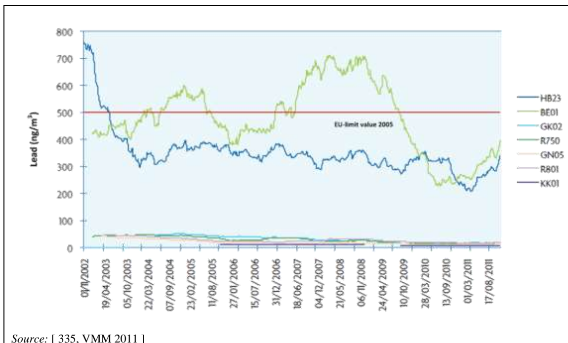
Figure 13.30: The trend in lead concentrations in PM 10 from 2002 to 2011 for some sampling stations in Flanders
