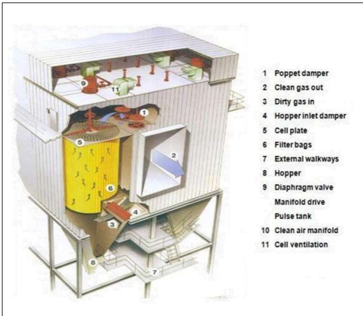
Figure 2.28: Low-pressure air pulsing cleaning system
