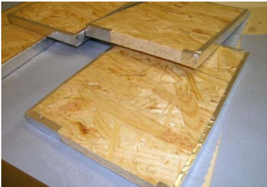
Figure 3-3: OSB prepared for chamber tests
