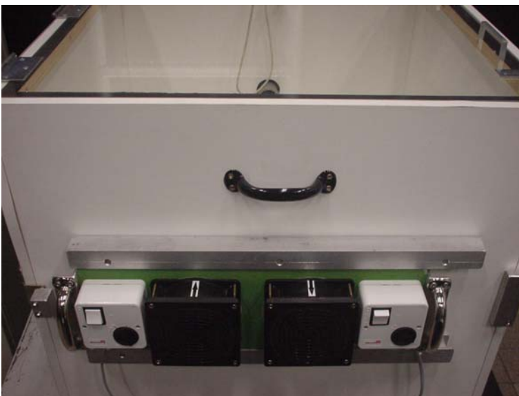
Fig. 11: View of the sampling device with the fans which can produce pressure or a vacuum in the casing
