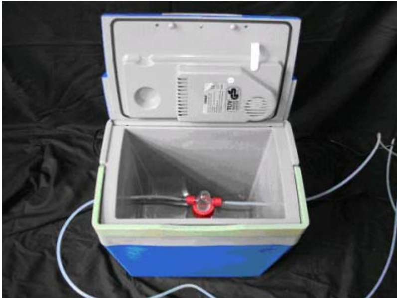
Figure 3: Constant source of acetone
