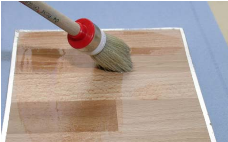
Figure 3-6: Application by brush of a lacquer on a wood carrier material
