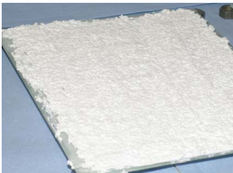
Figure 3-2: Synthetic-resin premixed plaster placed double-sided on a glass plate
