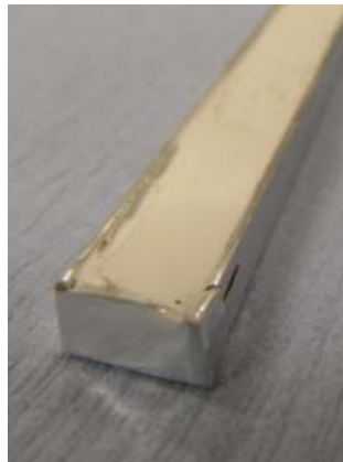
Figure 3-1: Applying sealing compound to an aluminium standard channel
