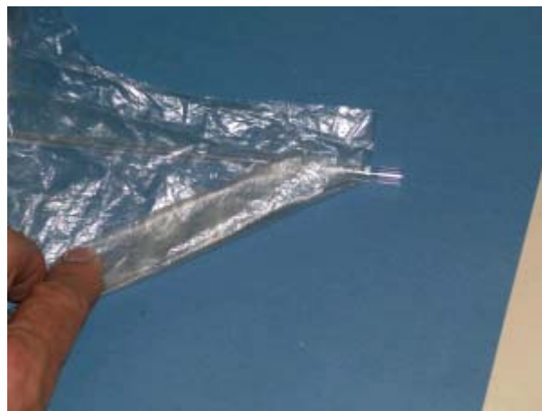
Folding the bag outlet towards the tube
