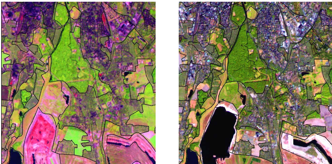
Figure 19: Improved satellite imagery for the interpretation procedure Comparison of Landsat 5 TM satellite imagery from 1990 (left), band combination 5,4,3 (RGB) and Landsat 7 ETM imagery, band combination 5, PAN, 3 (RGB). Depicted are subsets in the Southern Leipzig area.
