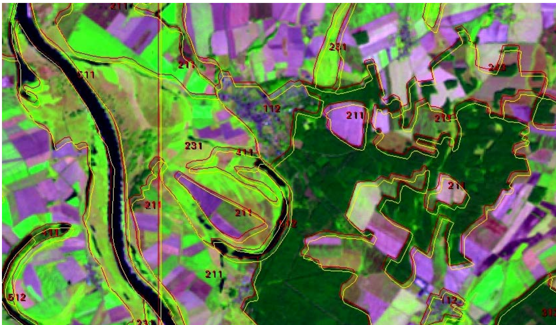
Figure 6: Example of the adjustment of CLC1990 vector data. CLC1990 polygons before the adjustment are depicted in yellow, polygons after the adjustment in red.
