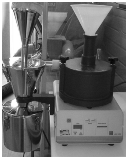
Figure 23: Centrifugal mill, Retsch ZM 1000.
