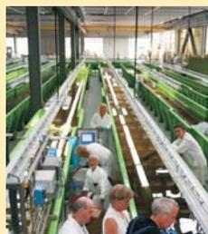
Figure 1: Indoor stream mesocosm system 106 m length, 1 m width, run in circular mode [5]
