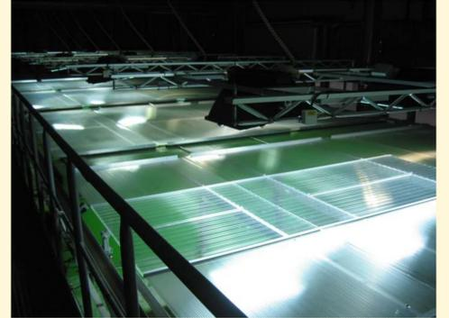
Fig. 1: Indoor pond systems (FSA) of the UBA with BFR-free plastics covers to prevent dust immission into the mesocosm system
