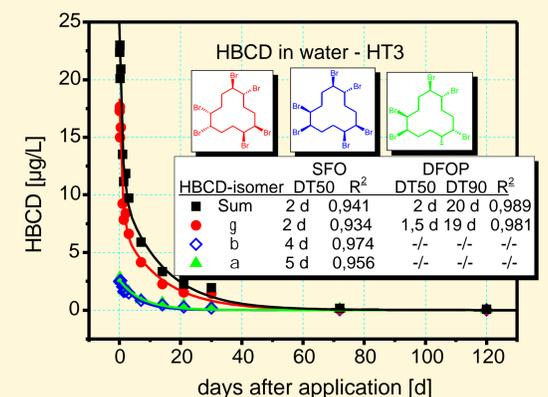
Fig. 5: HBCD (isomers + sum) - water concentration and DT50 in the spiked pond (HT3)
