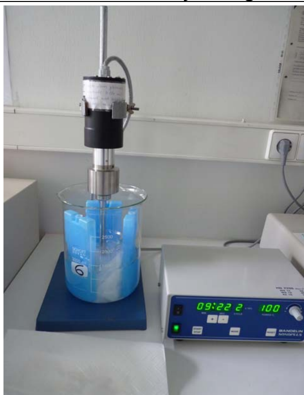
Figure 73: Preparation of the TiO 2 suspension.
