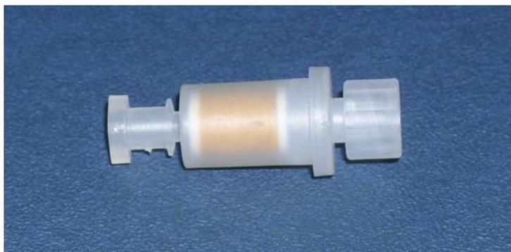
**Figure 4-23: DNP sampling cartridge for aldehydes and ketones**
