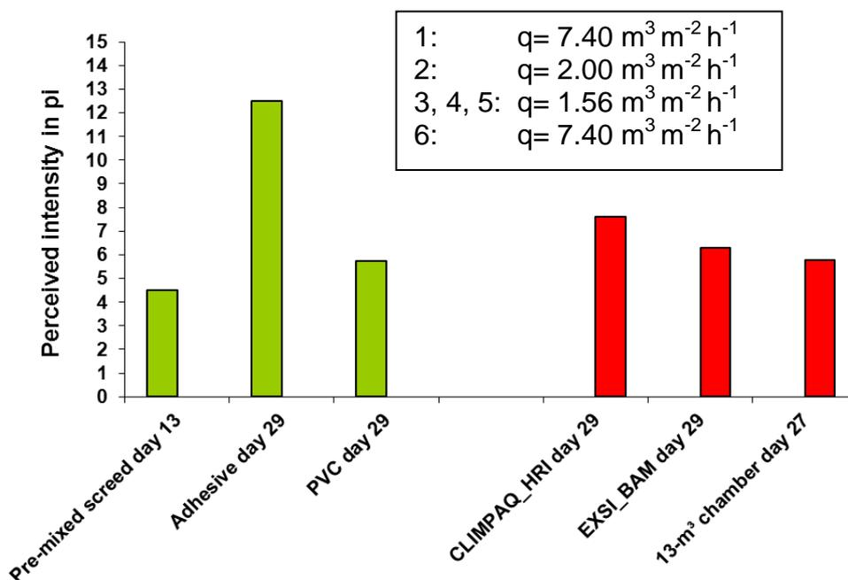
**Figure 5-43: Test results for a combination of building products (pre-mixed screed, floor covering adhesive, PVC)**
