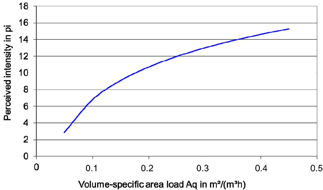
**Figure 6-5: Dilution characteristic of a building product (carpet); volume-specific area load ( $A_q$ ) as a function of perceived intensity of the building material**
