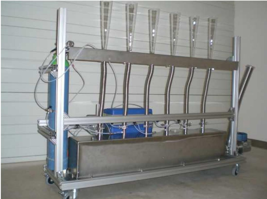
**Figure 5-27: Photograph of the simplified comparative scale**
