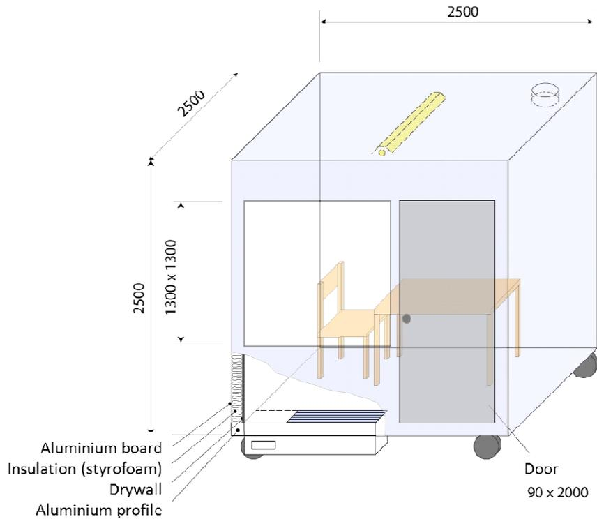
**Figure 4-9: Scheme of the 13-m<sup>3</sup> chamber**
