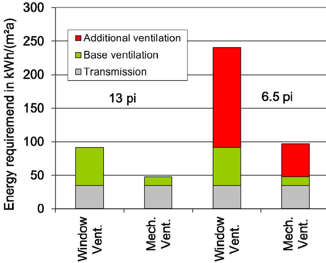
Figure 6-6: Surplus energy requirement due to increased air exchange caused by odorous substances in the room
