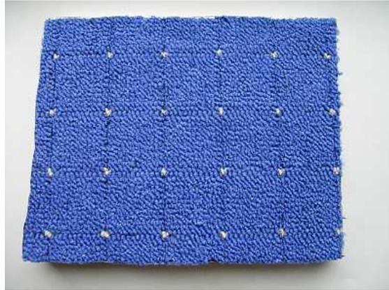
**Figure 4-13: Wall-to-wall carpet tailored for chamber tests**
