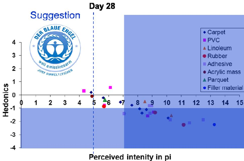
**Figure 6-2: Suggestion for the sensory-based limits for Blue Engel criteria**
