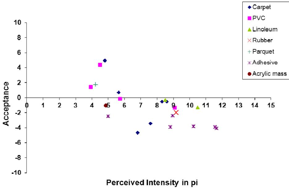
**Figure 5-6: Relationship between perceived intensity and acceptance for building products (in CLIMPAQ) on day 29**
