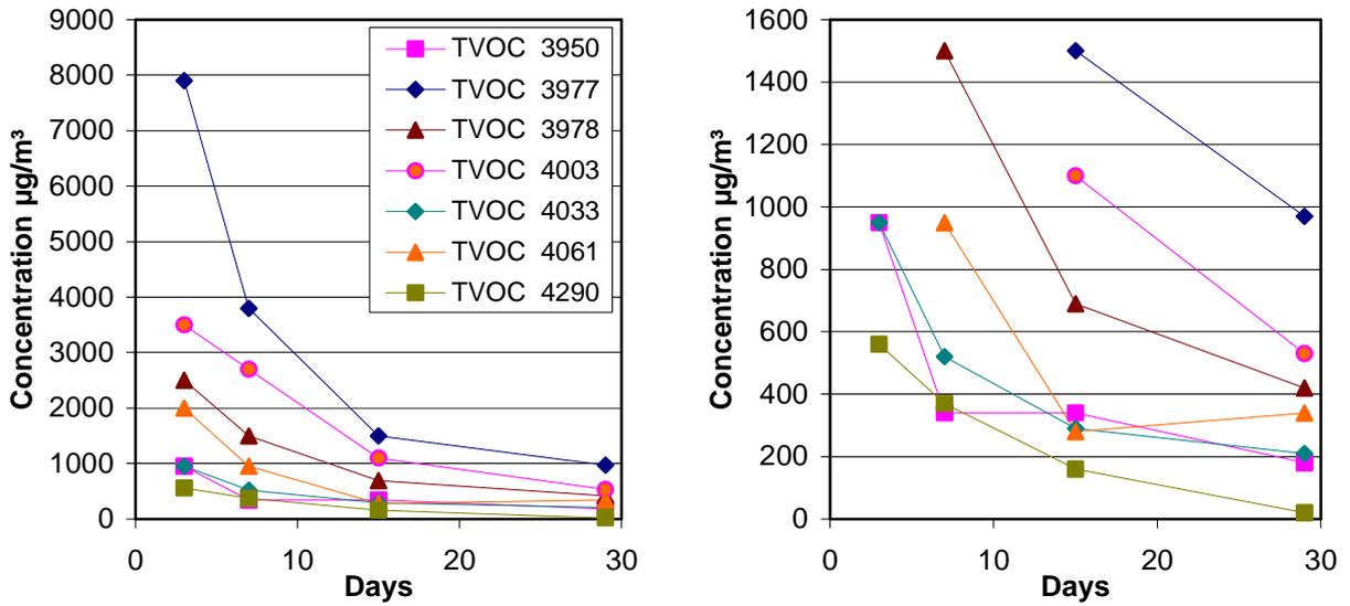
**Figure 5-20: TVOC concentration as a function of time for floor covering adhesives tested in the project (Diagram B is an enlargement of an excerpt from A)**
