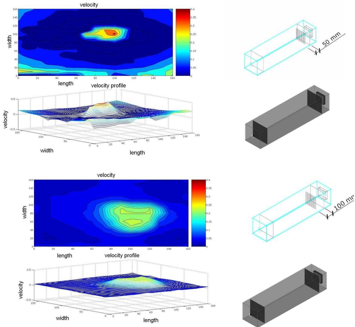
**Figure 5-35: Flow profile in the CLIMPAQ at a distance of 50 cm and 100 cm from the laminariser**
