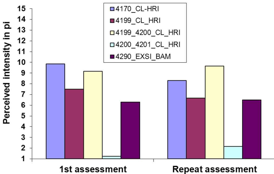
**Figure 5-31: Repeatability of the assessment of three individual building products and two combinations**
