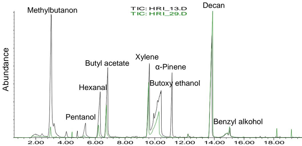
**Figure 5-25: Permeation behaviour of the PE foil (GC/MS chromatogram)**
