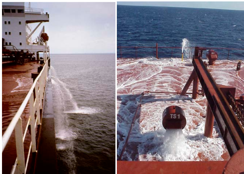
Figure 9: Open ocean exchange of ballast water. A. Ship undergoing mid-ocean ballast water exchange; B. Ballast water is forced out an opening at the top of the ship in flow-through exchange. (photos: Marine Invasions Research Laboratory, Smithsonian Environmental Research Centre. http://www.serc.si.edu/labs/marine_invasions/index.aspx )
