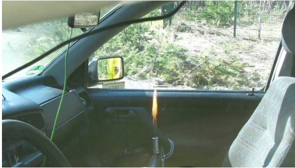
Fig. 20: Open flame of a small torch lamp operated with propane in order to ignite a leakage stream of HFO1234yf
