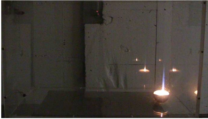
Fig. 12: Picture from the blue stagnant flame taken after 300 s from test no. V 04: release of HFO1234yf
