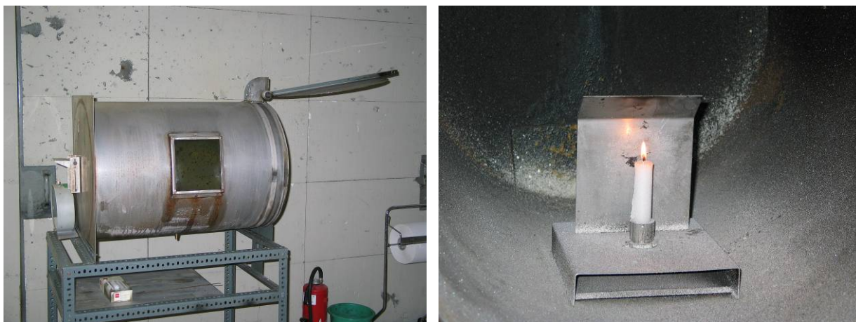
Fig. 14: Pictures of the set-up for the enclosed space ignition test (left picture: full view of enclosed space with open lid for pressure release; right picture: burning candle as ignition source)
