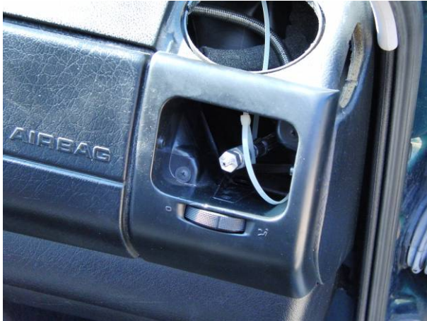
Fig. 18: Leakage pipe with a reduction part (inner diameter: 2 mm) installed in the ventilation slot of the front passenger
