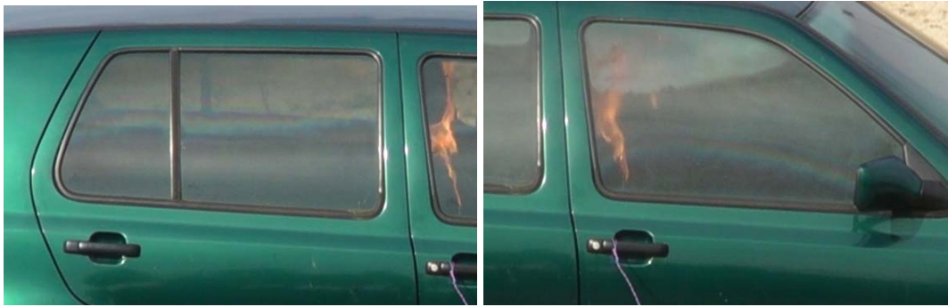
Fig. 26: Enhancement of two pictures shown in Fig. 25 (first two pictures of the second row) in order to demonstrate the translucent glass as a matter of the HF corrosion 50 s resp. 52 s after the ignition started.
