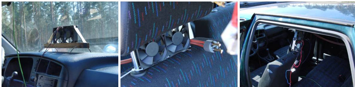
Fig. 23: Location of the fans for mixture homogenization
