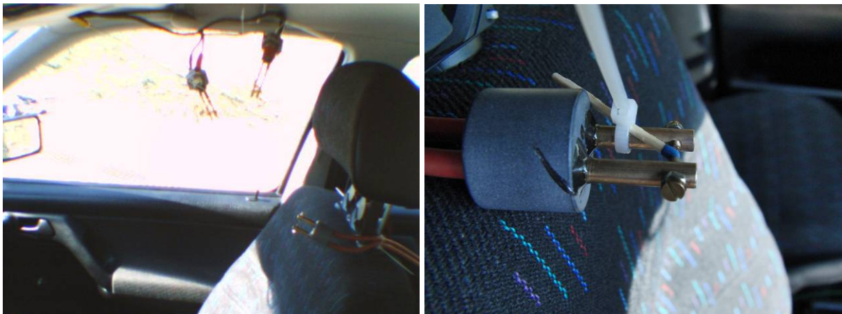
Fig. 19: Location of ignition sources in order to ignite a leakage stream of HFO1234yf (left picture: high voltage spark and “exploding wire”; right picture: modified high voltage spark for the ignition of a match)
