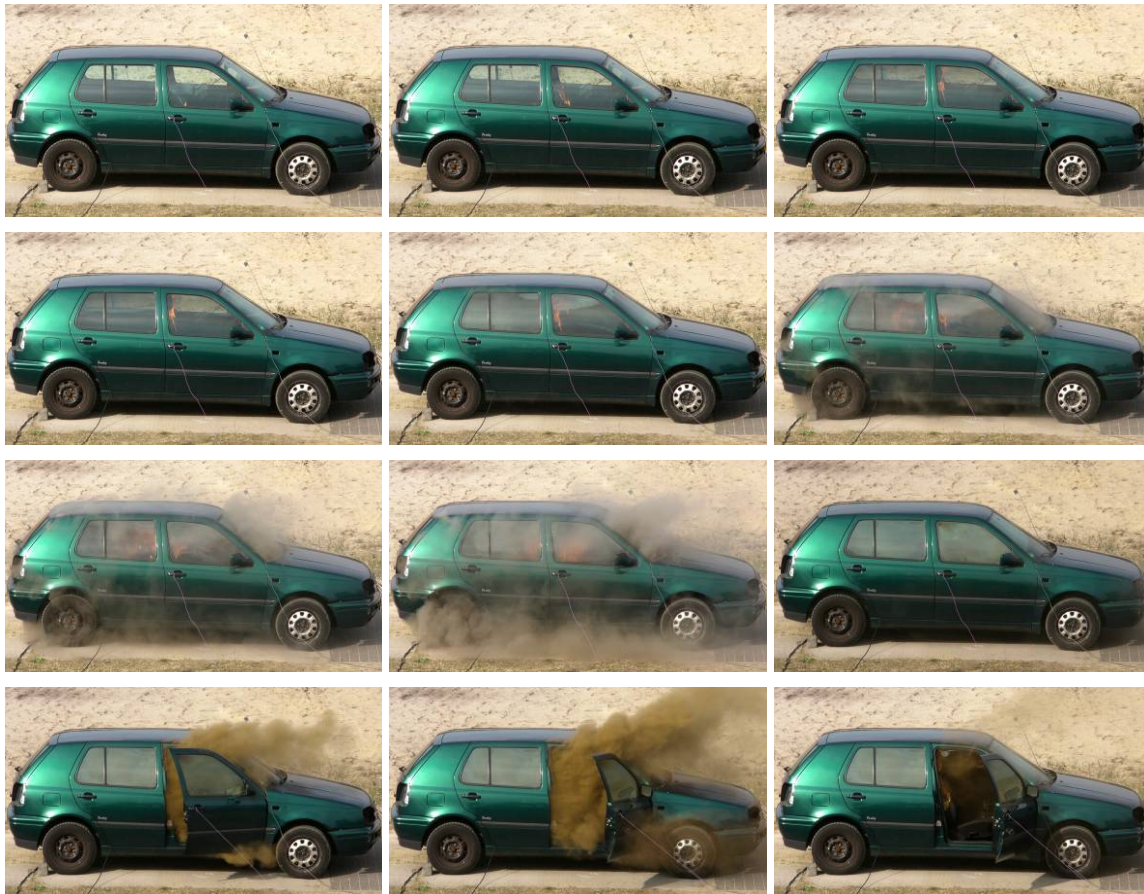
Fig. 25: Picture sequence from the video record of the ignition inside the passenger compartment.
