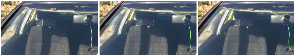
Fig. 24: Picture sequence from the video record where a HFO1234yf stream was ignited by use of a modified high voltage spark igniter with a match
