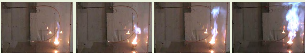
Pic. 3: Release of 46 grams of R 1234yf in 70 seconds with formation of hydrogen fluoride (HF) at levels above 90 ppm (© UBA 2010)(14)
