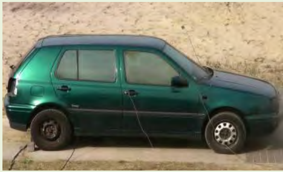
Pic. 4: Test car with windows etched by the reaction product hydrogen fluoride formed from R 1234yf during a fire in the car (© UBA 2010)(14)
