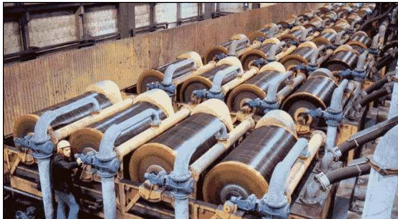
Figure 2.17: Low-intensity drum separators
