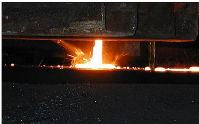
**Figure 2.24: Inoculation during pouring**
