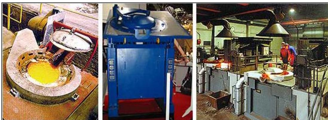
**Figure 2.14: Coreless induction furnaces [237, HUT, 2003]**
