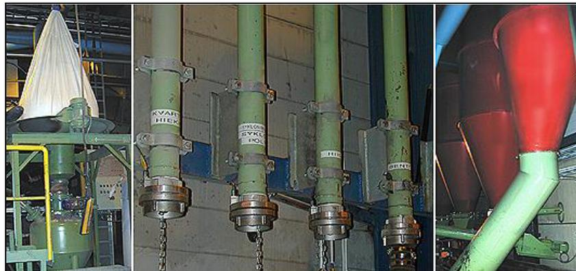
**Figure 2.8: Pneumatic conveyors and silos for powdered materials**
