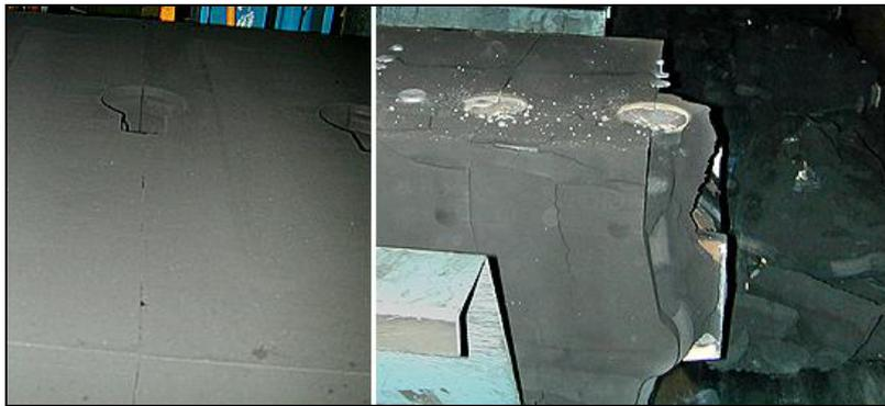
**Figure 2.43: Shake-out at the end of an automated moulding line**
