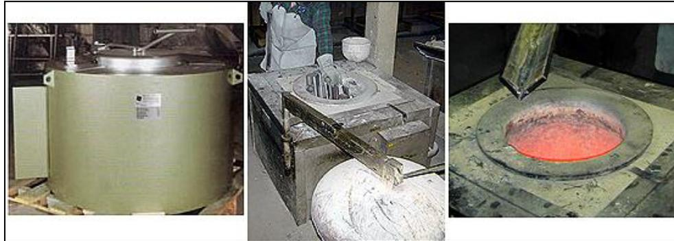
**Figure 2.20: Crucible furnaces**
