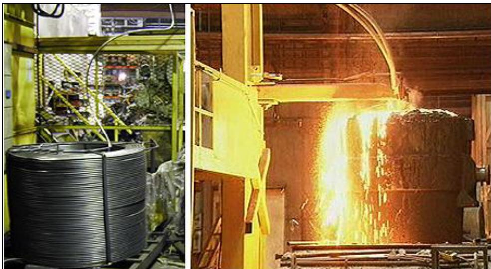
Figure 2.22: Deoxidation, using an aluminium wire
