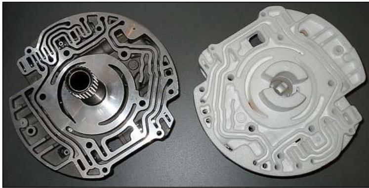
**Figure 2.37: Expendable polystyrene pattern (r.) for the Lost Foam process and an example of a casting produced by the Lost Foam method (l.)**
