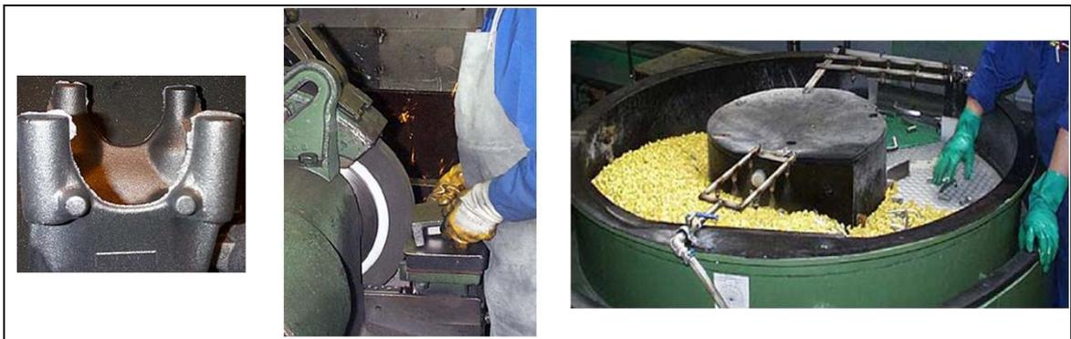
**Figure 2.51: Burrs (l.) and their removal using a grinding stone (m.) and slide grinding (r.)**
