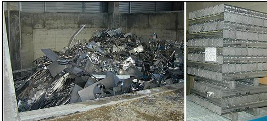
**Figure 2.7: Aluminium scrap(l.) and ingots (r.)**
