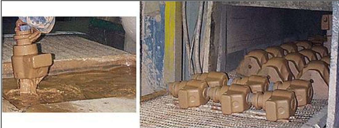
**Figure 2.35: Dip-coating with water-based coatings, followed by drying in a hot-air furnace**
