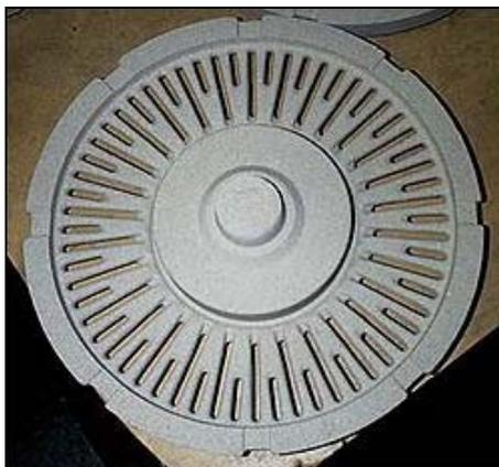
**Figure 2.32: Cold-box core**
