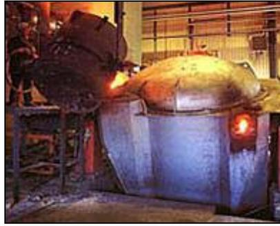
**Figure 2.16: Channel induction furnace**
