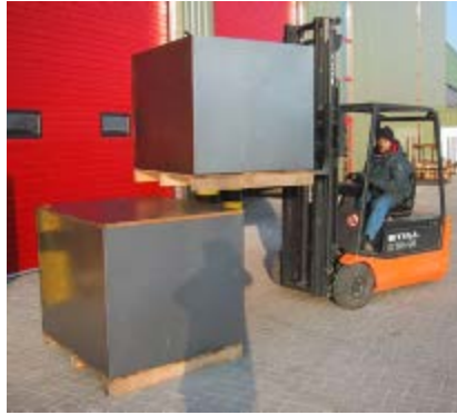
Fig. 15: Steel containers for the transportation and disposal of waste in underground landfills (© mh Verpackungsservice38)
