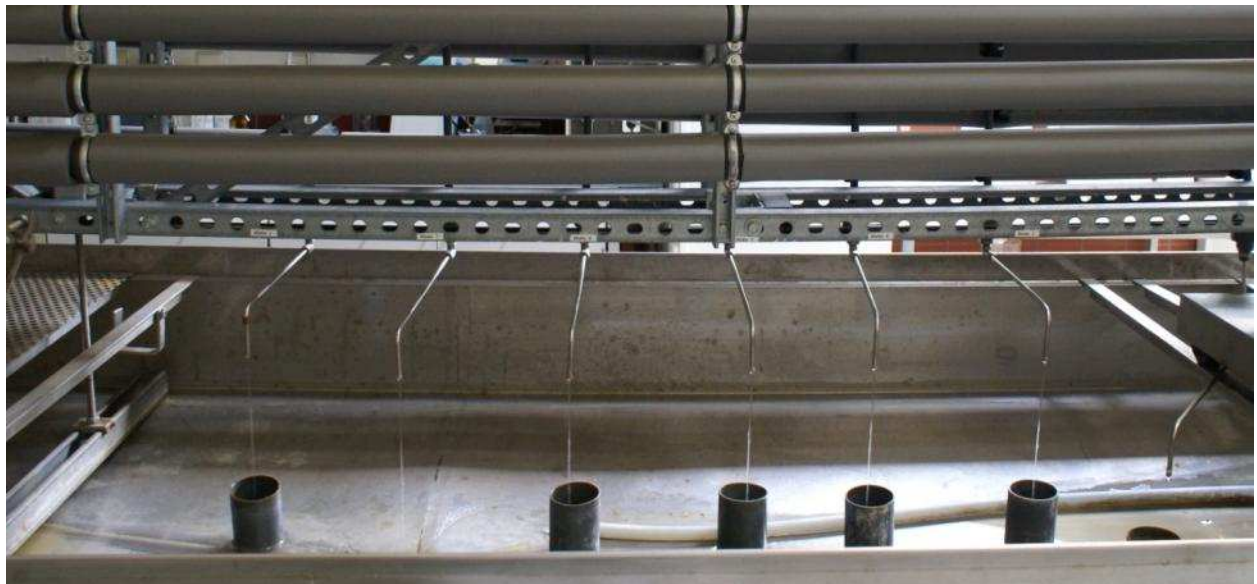
Figure 1b) Taps are small additional pipes. For the efficacy test stipulated in this guideline tap 0, tap 1, tap 2 and tap 3 are needed. Further taps to describe efficacy kinetics more precisely are recommended. After passing the rig, test water is discarded (flow-through mode).
