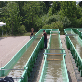
Figure 1: Stream mesocosm used for this experiment. The frames are suspending logs over the four pools present in the mesocosm
