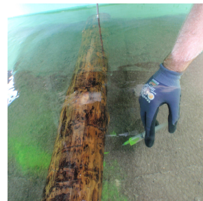
Figure 4: Use of uranine to illustrate vertical flux of surface waters
